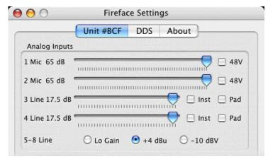
via the rotary encoder, or via the Settings dialog. The current gain is displayed in dB left to the fader. Further information is found in chapter 27.3.
