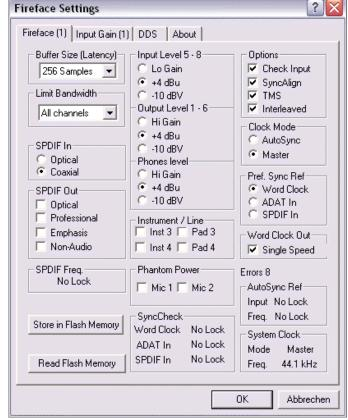
digital signals. SyncCheck indicates whether there is a valid signal (Lock, No Lock) for each input (Word Clock, ADAT, SPDIF), or if there is a valid and synchronous signal (Sync). The AutoSync Ref display shows the input and frequency of the current sync source.
