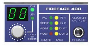
**Phones** is a low impedance line output of highest quality. It provides a sufficient and undistorted volume even when used with headphones.
