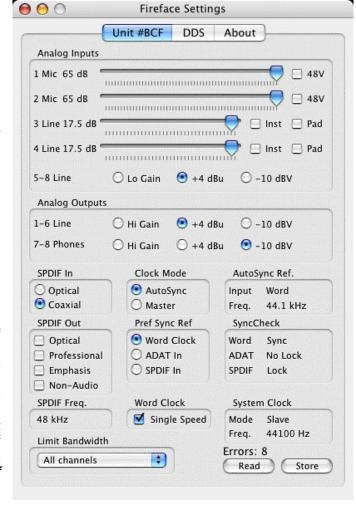
The string **Errors** is displayed only when transmission errors of PCI/FireWire are detected. The display will be reset on any start of a playback/record, i.e. set to zero and is thus no longer visible. More information can be found in chapter 37.3.
