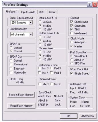
standard frequencies, but also any sample rate between 28 and 200 kHz. Even the word clock input, most often used in varispeed operation, allows any frequency between 28 kHz and 200 kHz.
